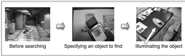
(a) Usage of the prototype (in the case of finding an object without occlusion)
