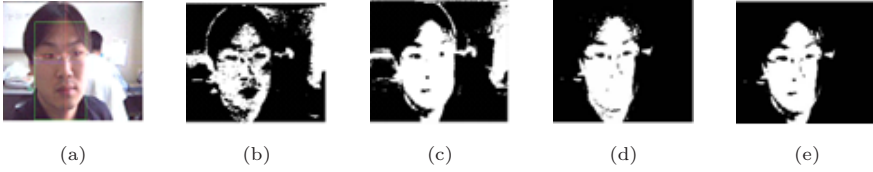
Fig. 1. Facial skin color detection in daylight; (a) Original image, (b) resulting image using H component, (c) Cr component, (d) I component, (e) multi-color model
