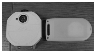
Fig. 4. Ultrasonic Tag (left) and ActiveRFID Tag (right)
