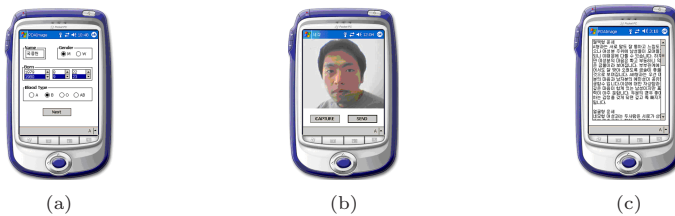
Fig. 11. Proposed face analysis and automatic facial avatar drawing system based on PDA; (a) Initial page, (b) face detection, and (c) facial physiognomy analysis
